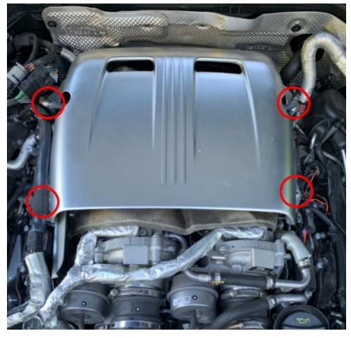
9. Remove OEM heat shield by unscrewing 7 x E10 bolts
