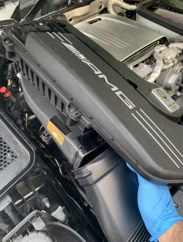
7. Pull up on the driver side airbox to release them from the ball-studs.
