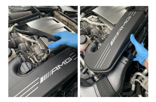
8. Remove outer silver turbo cover by unscrewing 4 X 10mm nuts. You will need a 10mm open wrench to hold the stud in place.
