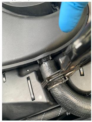
5. Loosen turbo clamp connectors on both sides.
