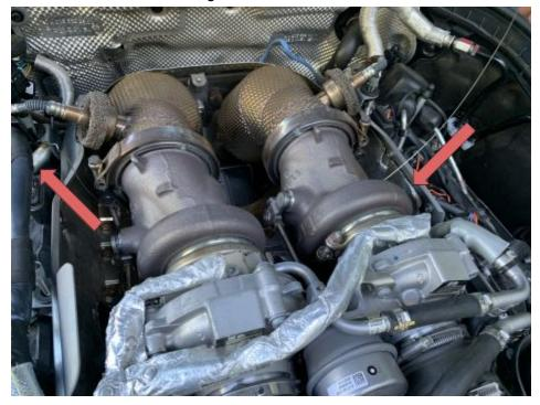
11. Once these are in place, lay the blanket down and loop the passenger side tie wires to the rivet, leaving little to no slack.
