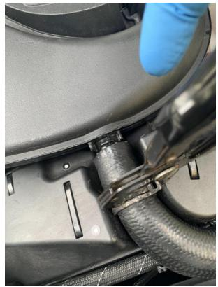
5. Loosen turbo clamp connectors on both sides.
