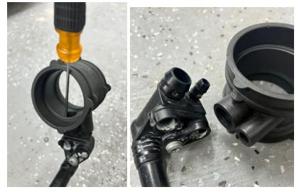
9. After it is loose, separate the OEM couplers and replace them with the new larger couplers. If your vehicle has 3 ports on the recirculation body, remove the plug that comes pre-installed on the upgraded coupler.
