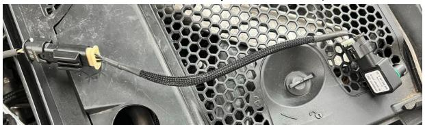
14. Install the sensor into the intake tube and ¼ turn it to secure it in place
