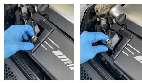
3. Remove both sensors and set them aside to be placed into the new intake.
