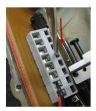
3. As you continue to press down, push the screwdriver towards the housing and the terminal block will open.
