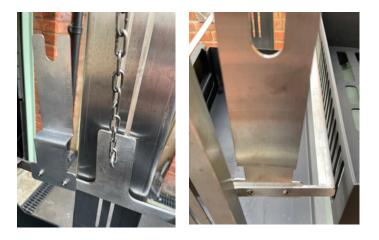
**Step 3** If you have not already slide the motor into position on the left hand bracket as in the picture above
