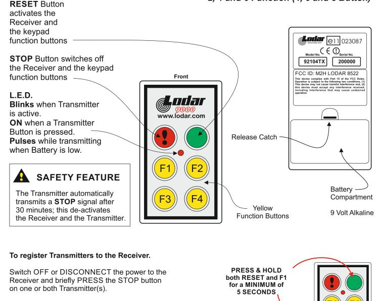
Switch ON or Reconnect the power to the Receiver. This opens a 20 second registration window in the Receiver processor.
