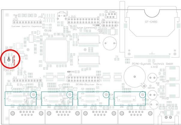
Position of the rotary switch for the Router ID
