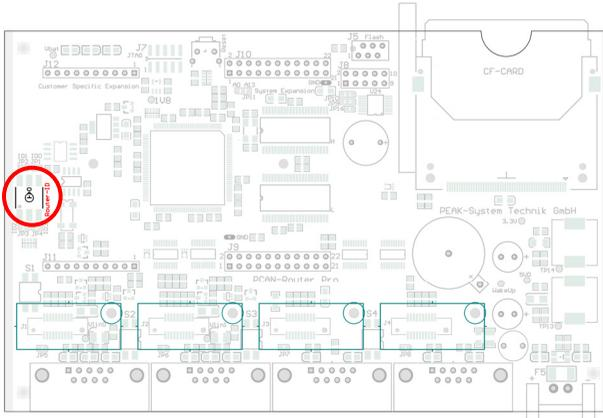
Position of the rotary switch on the circuit board of the PCAN-Router Pro
