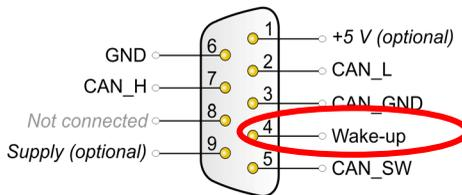
Wake-up pin 4 at ports CAN 3 and CAN 4
