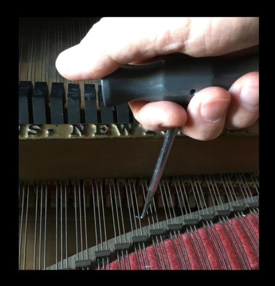
Place 200g weight on bass string #3 as weighted kissing sample will otherwise push this flexible string up slightly before "letting off" causing a measuring error.
