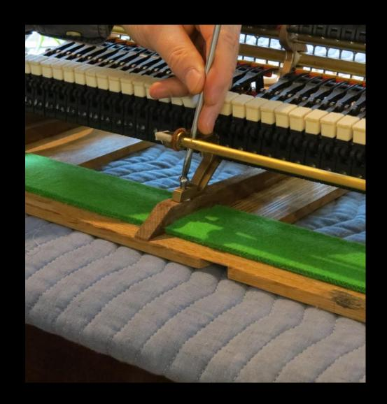
Check frontrail bedding, holding down manually for crowned frontrail. If areas tap back, sand no-tap areas with strips of sandpaper grit side up until none tap.
