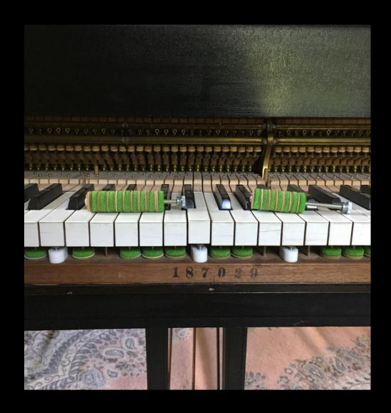
Move keyframe for strike sampling so hammer wearmark "valleys" are between strings (Regulating Rack templates can only touch "hills").
