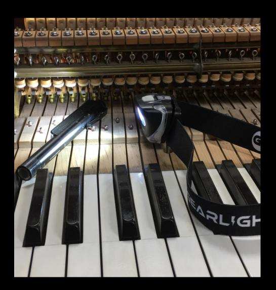
Regulate natural backchecks as high as possible (no tail scraping when hammer is played against a resistance).
