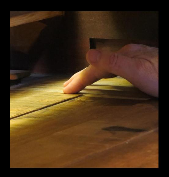
Check out keybed shape for flatness or lack of flatness side-to-side and front-to-back to know what to expect during bench setup.
