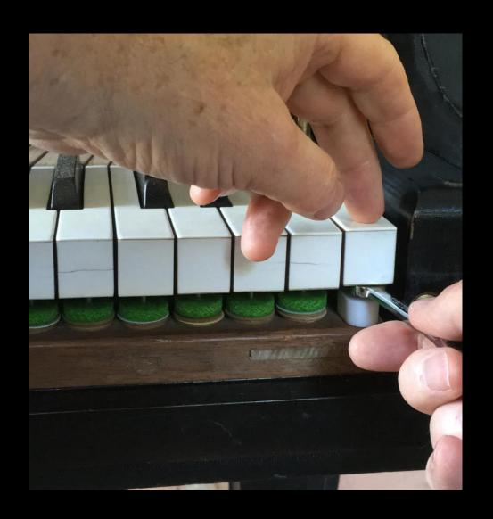
Lift key #44 with its Keystep to just contact straightedge supported by preleveled end keys this memorizes overall shape of frontrail.
