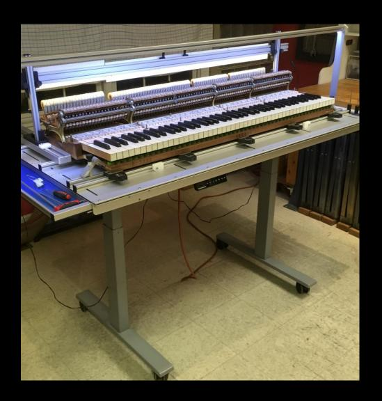
The Full Monte also includes Action Tray, Work Tray, and Hammer Hanging Jig (which works from the Squaring Platform).
