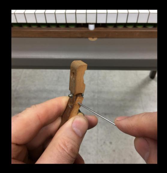
Firmly work parts to make stable – apply pressure with pin against part of cloth manipulated (number of swings can be cut in half).
