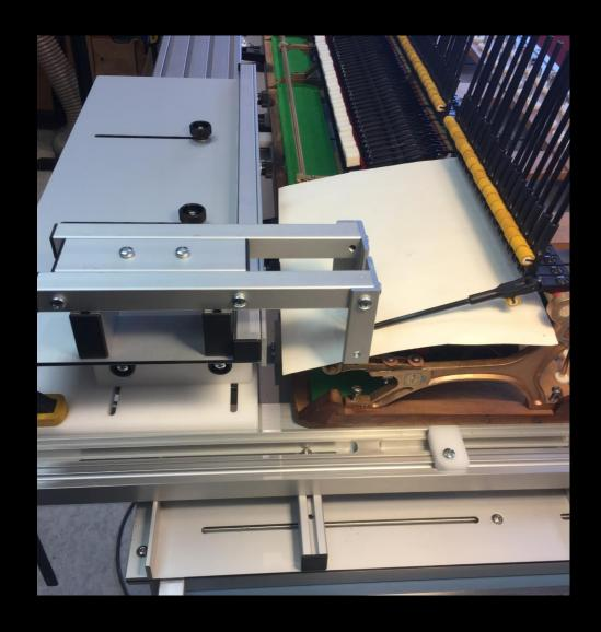
The Shank Traveler provides reference edges for traveling shanks to vertical (touch shank to a reference edge to add tactile and aural referencing to the visual).
