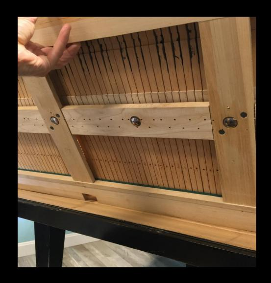
Check bedding with action fully assembled – test backrail with long screwdriver through strings on rest cloth over contact lip.
