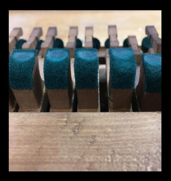
After adding pad treatment and smoothing/compressing with flat iron on wool setting, they are like new.
