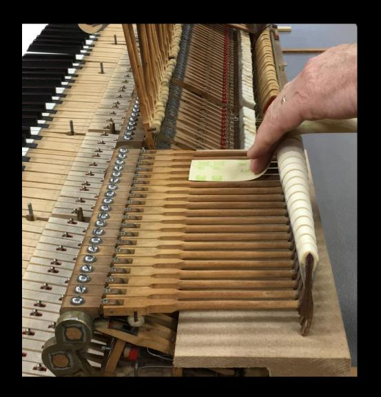
The SFV Block can also offer a solid surface to support hammers for voicing, and it is wide enough to span most sections.
