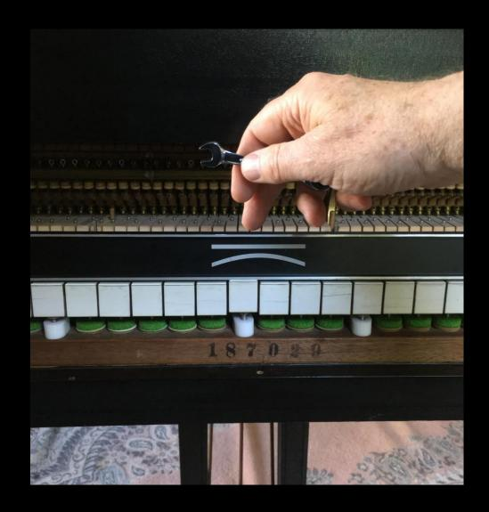
Remove front punchings from strike samples (end-of-section naturals but not bedding samples) to other machine screw as extra aftertouch will be needed.
