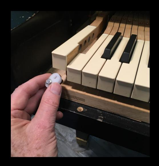
Pre-level keys #1 and #88 (or #85) with cut punchings — wait for sharps until action is set up on bench.
