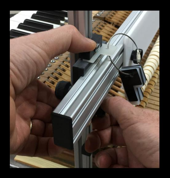
Setup takes seconds and perfectly tapers letoff from one end to the other.
