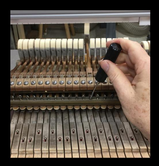
Regulate a sample so jack tender and rep lever engage letoff button and drop screw simultaneously and regulate the rest to the resulting symptom.
