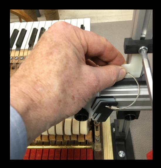
Lightly clamp strips (with the least pressure that will work) to hold down frontrail by guide pins.
