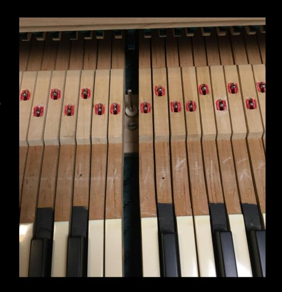
Friction affects sampling so, if necessary, take action apart to ease keys, lubricate centers, and space for clearance.
