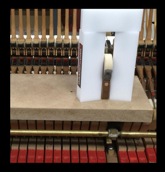
For hammers that require tilting for clearance, add a stilt. Avoid this if possible, however, for better tone, power, repetition, and stability.
