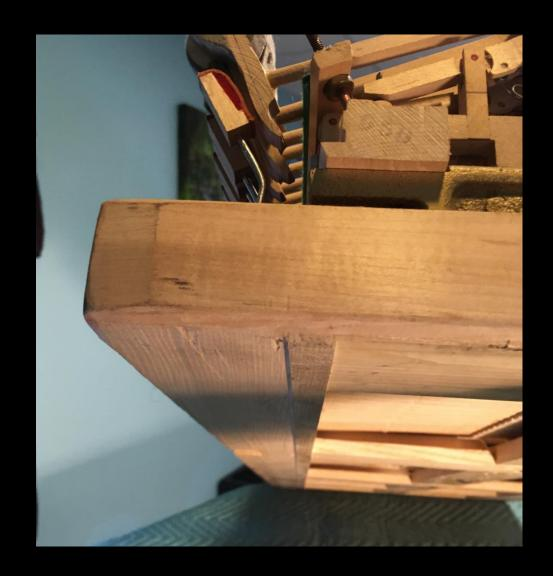
If backrail needs bedding, remove keys and topstack, sand areas of contact until full contact (or consider balance punching shims under topstack feet to complete fit).
