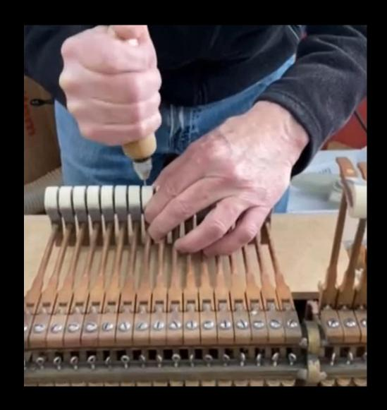
Squaring, spacing, and leveling keys are easier on the bench (use topstack not weights for the fastest route to best key leveling).
