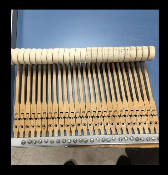
Adjust friction in hammer flange centers while hammers are off topstack (and repin repetition levers as needed if whippens are off too).
