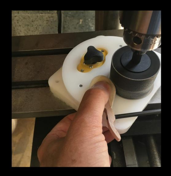
The Filing Jig makes getting consistent size and shape easy — wait to gang-file straight-bored hammers on SFV Block when reassembled.
