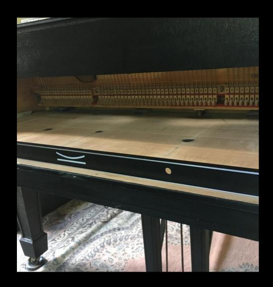
Turn up glidebolts and bed cheek blocks to bring rail to keybed but not over-bear on guide pins – remove factory shims/shim or adjust brass fittings/shim cheek blocks as needed.
