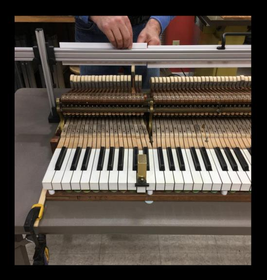
Add strips to stop Regulating Rack where crowns of hammers touch templates at strike – all regulating happens from there back.
