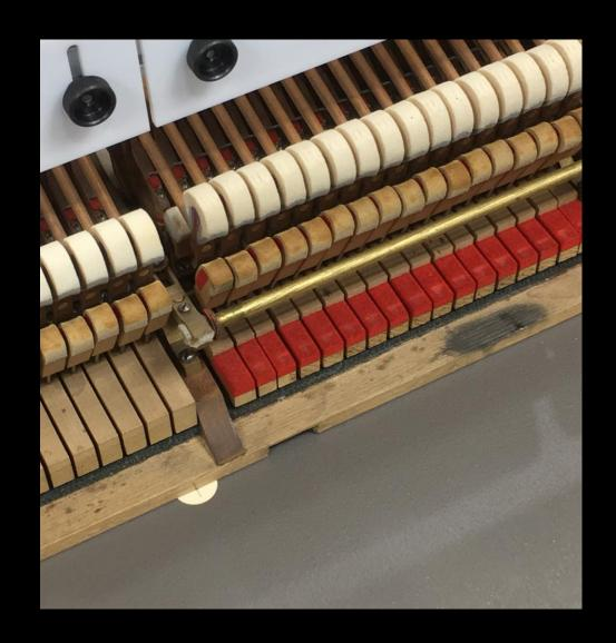
Shim frontrail (lift rail for punching insertion with tapered felt knife) so that key #44 just touches straightedge — test three points of contact.
