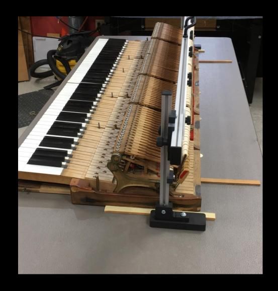
Select Regulating Rack templates that extend slightly beyond hammer sections (use two templates butted together for long tenor section).
