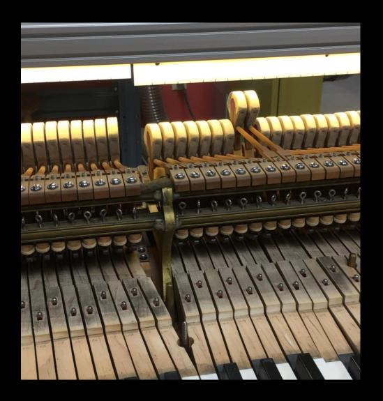
Check backchecking accuracy every so often with Gauge Key (narrow widths offer incremental backchecking distances) and touch up as needed.
