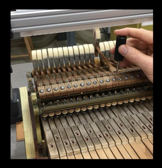
Lower rail to stops and regulate hammerline – sight with Regulating Rack just slightly back to reveal hammers that overshoot.
