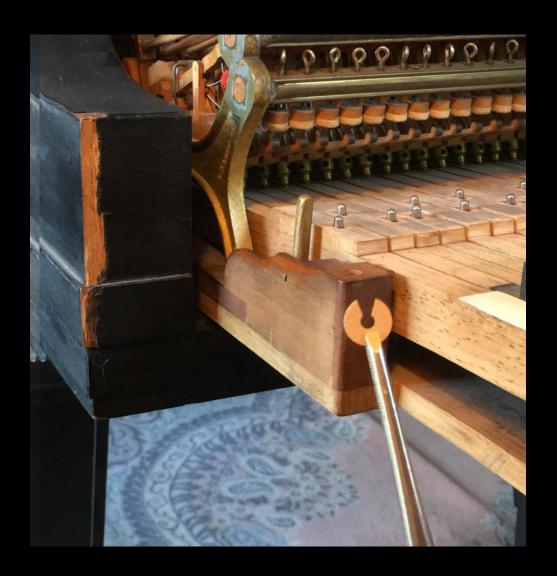
Make sure straightedge clears all keys. This will mean raising level of end keys even if not leveling (just remove punchings after setup).
