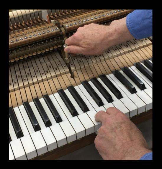
Block weighted samples of strike with templates and fine tune template heights so keys hesitate and drop like they did in the piano.
