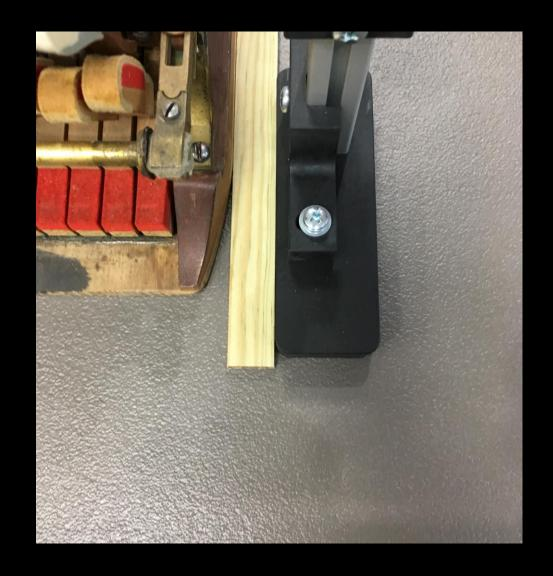
Add two strips at back as stops for front-to-back positioning. Now action can be removed and returned to exactly the same place.
