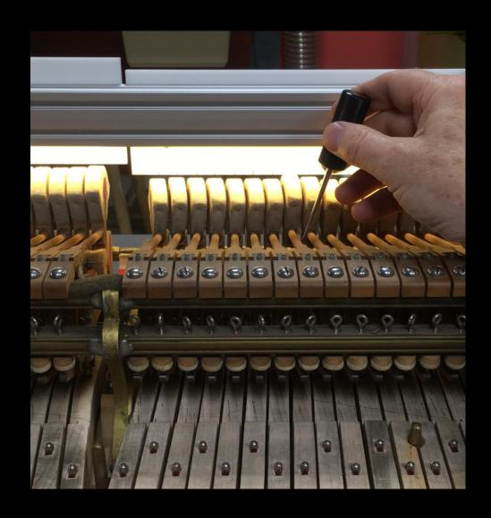
Return rail to strike and regulate aftertouch one-ata-time and in clusters, refining by adjusting dip, letoff, and drop.
