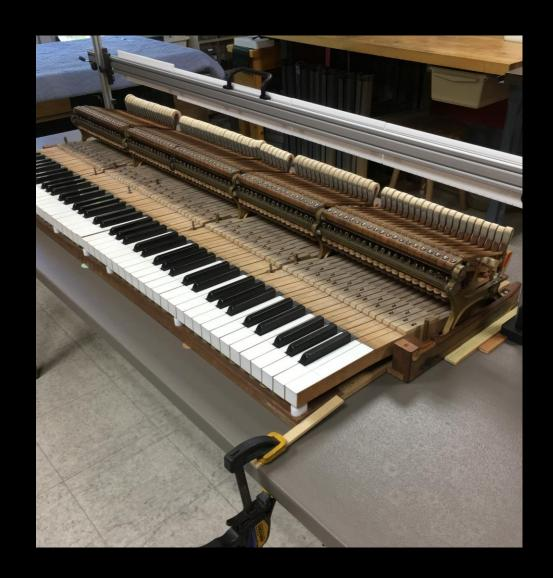
Grandwork Tools now offers a kit to help fix the position of a grand action (its tape has strong adhesion but is easier to remove than most when finished).
