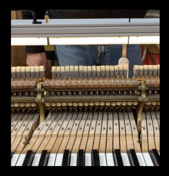
With dots in registration holes, the Underlevel/String Height Gauge records five strike heights per side of plunger — more accurate than numbers.
