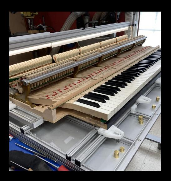
Note outliers here (probably from varying friction in a downweight-only weighoff). Chalk zeros mark keys that are correct without adjustment).
