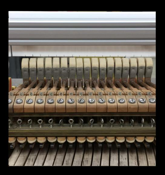
Set up hammers to be at strike for squaring to vertical with Hammer Square on SFV (squaring/filing/ voicing) Block.
