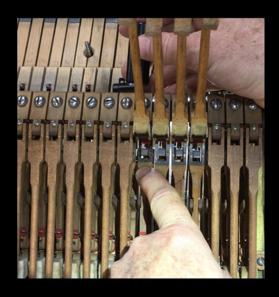
Then complete jack positioning with straightedge held sample-to-sample, sighting fronts of jack tips.
