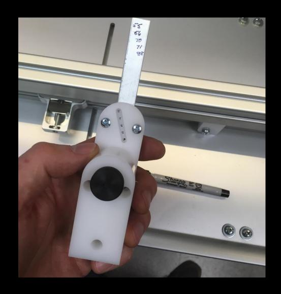
Remove hammers from topstack and file flared hammers on Filing Jig with firm pressure at tip of molding and slight sideways pressure into drum.
