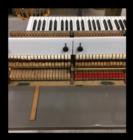
Set lower stops to touch underside of brackets and upper stops to be blow distance above brackets – the middle white Gauge Key is 1.75" long (others are shorter and longer).
