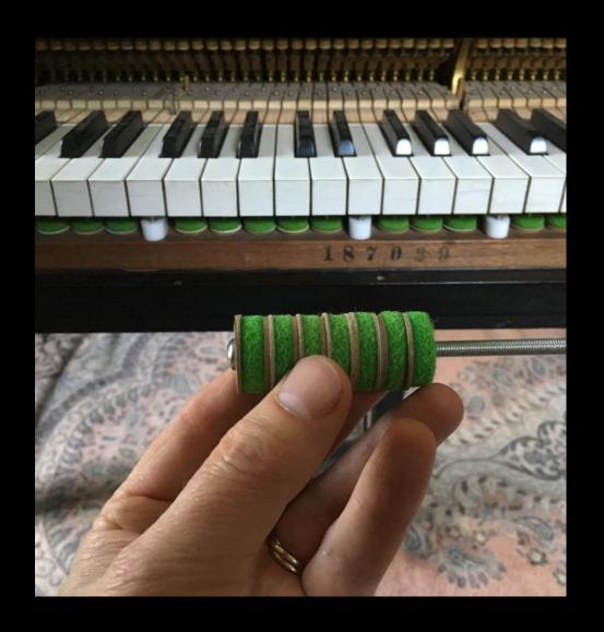
Choose from two sizes of Keysteps for fit under keys — note underside of Keystep slot has countersink to clear keypin shoulders.
