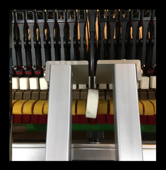
The Hammer Square on a Squaring Platform squares hammers to vertical at strike more easily and accurately than on a SFV Block.
