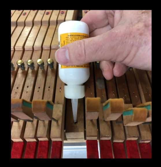
Watery hot hide glue sizes balance holes that backchuck and tightens more with multiple applications.
