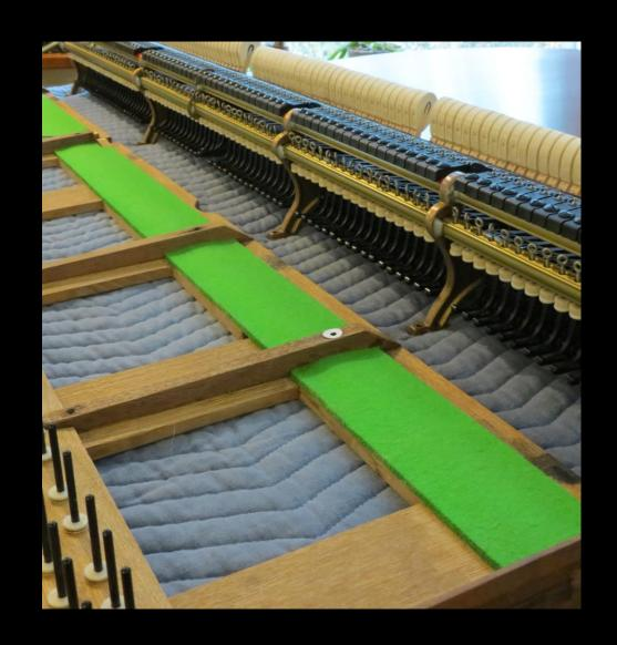
Glue punchings to cleats, clamp with topstack, and validate then trim as needed. Rule: if light touch on cleat completes backrail fit, shim.
