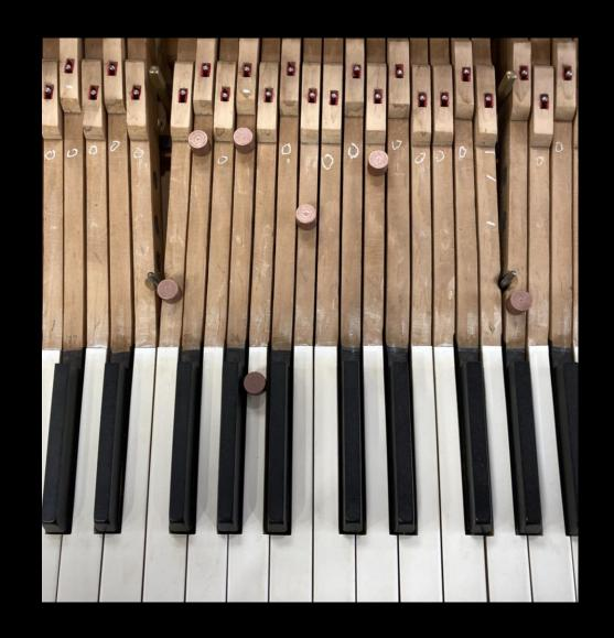
Returning action to piano, touch up balancerail bedding with pedals, re-install return spring, and square spring as needed.
