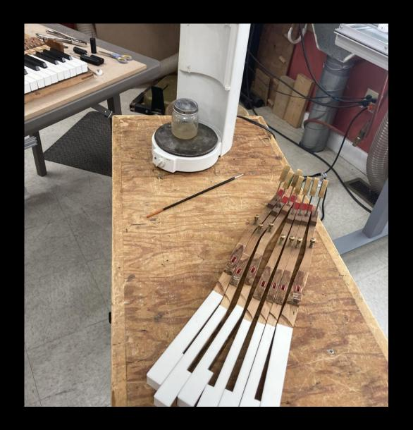
Use Gauge Keys (thinnest white for treble, thickest white for bass) to position Template Rail for letoff.
