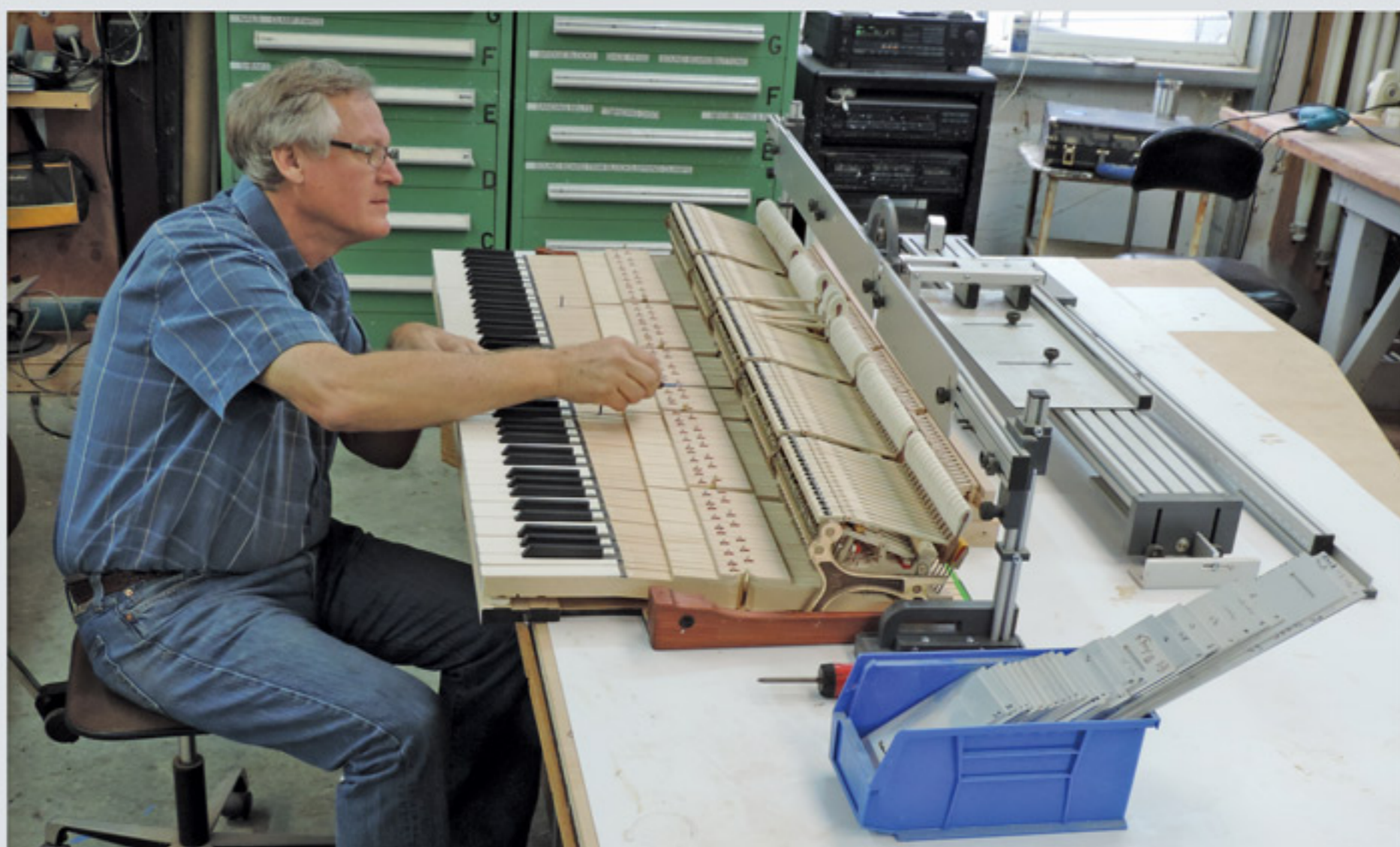
Putting the finishing touches on a custom balanced D action with the TPR tools
