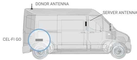
Find a good mounting location in your vehicle. Location should have airflow (*for cooling*) and be secure from contact with external objects. Make sure the unit is within cable range of the 12V power supply on your vehicle. Best to make sure all cable lengths support the intended mounting location BEFORE permanent mounting.
