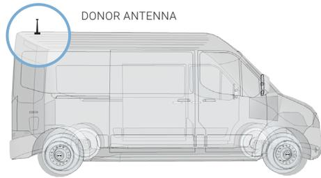
Place the Donor Antenna on the vehicle. Make sure you consider the entire system and required cable lengths.
