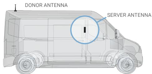
Install Server Antenna in the cab where coverage is needed.
