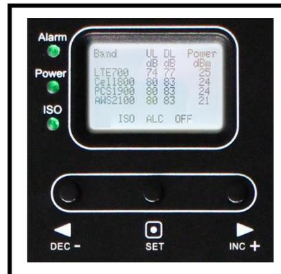
Professional LCD panel displays gain levels and output power in each band to enable easy setup, troubleshooting and outdoor / indoor antenna alignment and placement.
