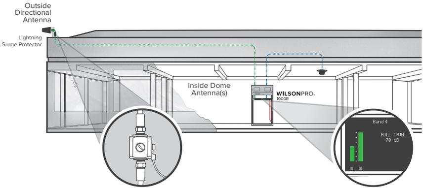
The direction of the outside antenna should be adjusted until the "DL" bar is maximized.
