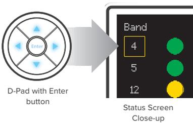
By pressing enter on a highlighted light, as shown, a more detailed status screen will be displayed for the highlighted band.
