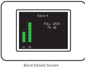
This screen provides specific band and port information. Including the strength of the received uplink and downlink signal, status details, and the amplifier gain.
