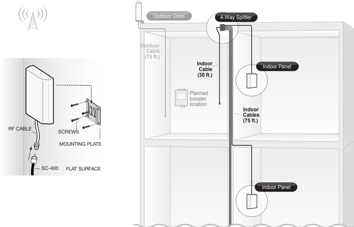
**Note:** If desired surface for installation plate is wood or concrete, wood or masonry screws for L-plate will have to be purchased separately.
