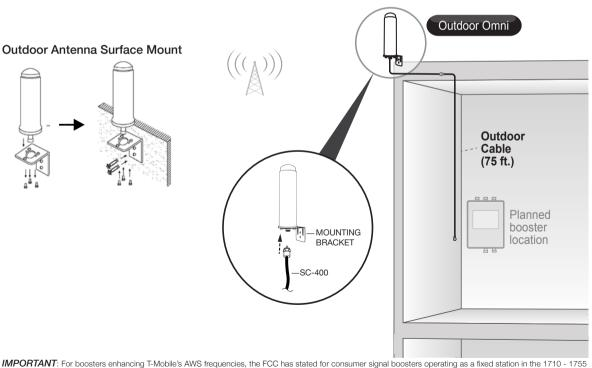
IMPORTANT: For boosters enhancing T-Mobile's AWS frequencies, the FCC has stated for consumer signal boosters operating as a fixed station in the 1710 - 1755 MHz uplink 2110 - 2155 downlink bands, the users or installation manual must contain the 30 foot height restriction requirements per FCC 27.50(d)(4)
