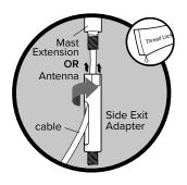
Add thread locker (packets provided) to thread point and screw on the **Side Exit Adapter.**
