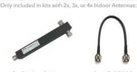
2x 2-Way, 3-Way, or 4-Way Signal Splitter
