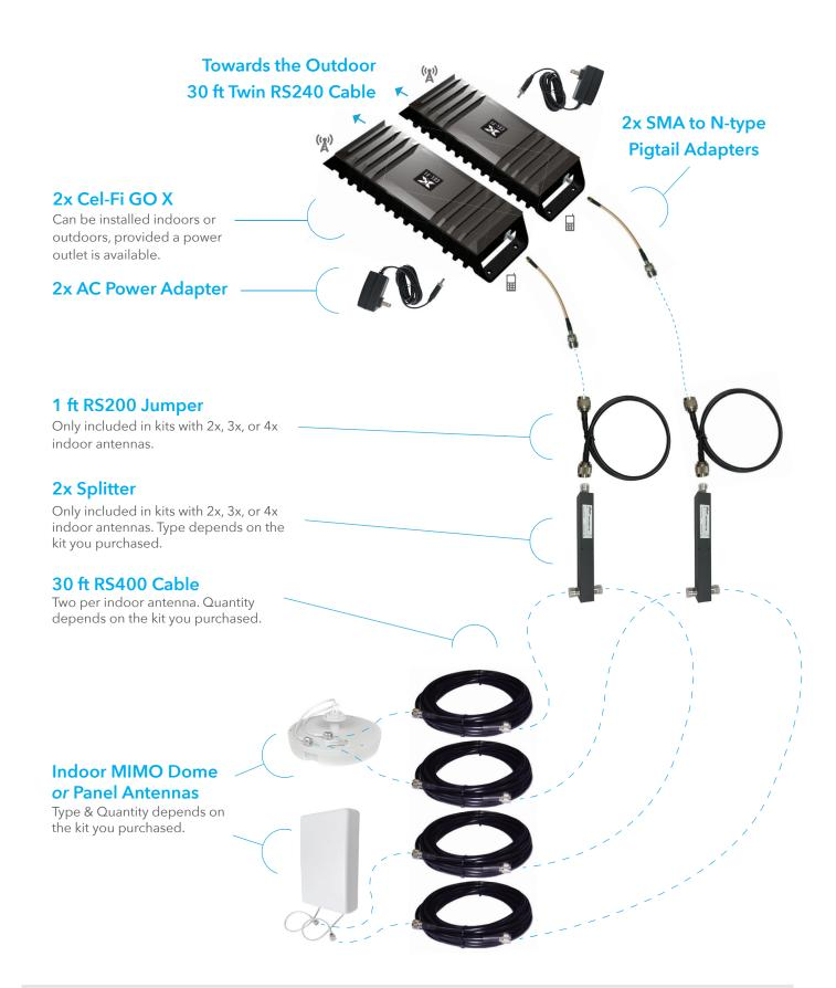
**Tip:** Make sure that the two cable paths for each indoor antenna connect to a different Cel-Fi GO X amplifier. If an indoor antenna has both cables paths connected to same Cel-Fi GO X, it will not broadcast a MIMO cell signal.
