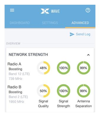
The most important information is summarized at the top of the screen, under the "Overview" section. The information here is divided into two "radios" - the GO X's two radios are what allow it to amplify up to two bands simultaneously.
