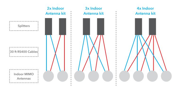
**Tip:** Use Painter's/Masking Tape to label the RS400 cables as "GO X #1" and "GO X #2" to keep track of which RS400 cables go to each Cel-Fi GO X.
