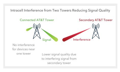
quality directly. However, by shielding and aiming the directional outdoor antenna that's included in your kit you can find higher quality signal, and the GO X's will amplify that signal and rebroadcast it indoors.
