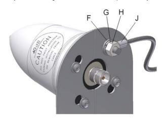
**Mount to Mast Assy** – position antenna onto Mounting structure. Route hose clamps and tighten 2X.
