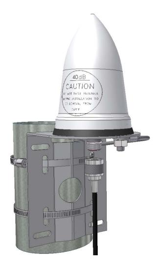
Attach the other end of grounding cable to shortest possible ground connection. Attach coax cable, and Install weatherproofing (not provided with the Mount Kit) extending at least 2" below the bottom of the connector to directly underneath the base plate of the antenna.
