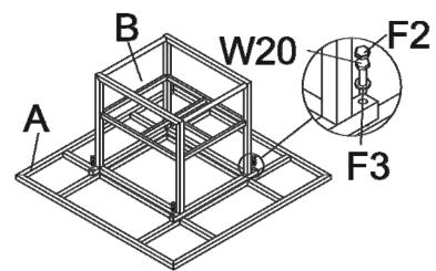
Before attaching the Bolt Head Covers, tighten all bolts with Spanner (S1).
