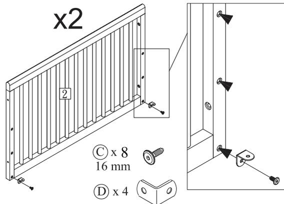
EN: Insert the angle brackets D and screws C for fitting mattress base in one of three height positions.
