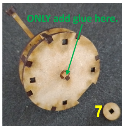
21: Glue the deck gun onto the weapon platform. ONLY add glue onto the squared tap, so that the gun can turn. Glue on part 7.
