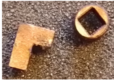
16: Glue together shown pieces for the ship's marker lights (x3). Front starboard (Green), Front port side (Red), Aft (White).
