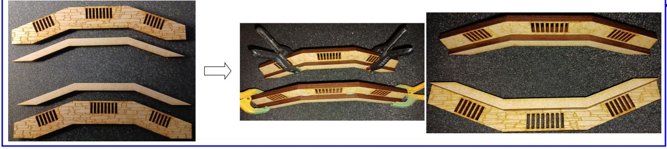
4: Glue together shown pieces, and use clamps until glue is dry. First glue on middle section, and let it dry. Then glue on the last two.
