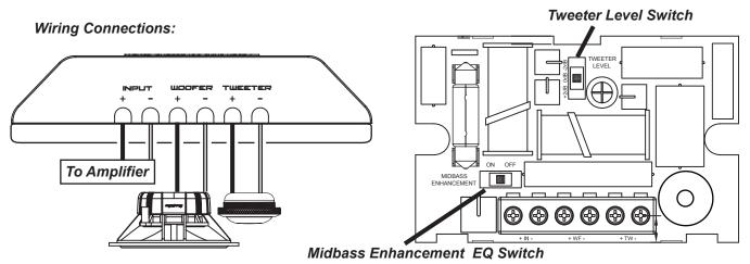
**Tweeter Protection:** Most component speakers offer a simple one stage "tweeter shut down" for protection. The Tl3x system provides two stages (polyswitch and lightbulb) that variably optimizes the signal to the tweeter when automatically activated. This protection system adapts to the dynamic signal level of the music, so it always provides just the "right" level of protection.
