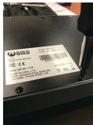
Remove the 6 cross head screws from the bottom side of the DSP8.8
