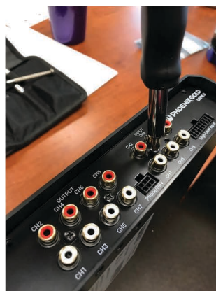
Remove the 6 cross head screws from the input side of the DSP8.8
