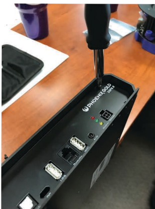
Remove 4 cross head screws from the remote interface side of the DSP8.8
