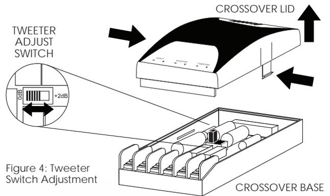
Figure 4: Tweeter Switch Adjustment
