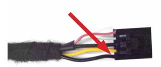
3. Flip the plug over and remove this wire by pressing on the release tab with a straight pick or similar tool.
