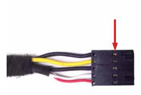
4. The plug should look like this when finished. Secure the wire with electrical tape and re-connect to the amplifier.
