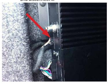
2. Locate the black wire in Pin 1 of the 5-pin plug.
