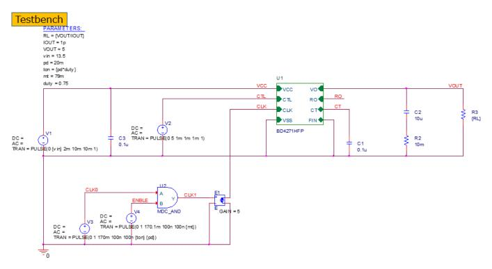
When WDT threshold Voltage VCLK is ON ⇔ OFF (Input=13.5V Output=5.0V IOUT=1pA)
