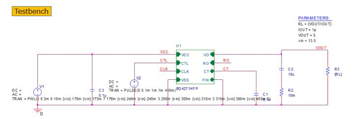
When supply voltage VCC is ON ⇔ OFF (Input=13.5V Output=5.0V IOUT=1pA)
