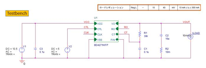
Load regulation (Input=13.5V Output=5.0V IOUT=10mA~300mA)
