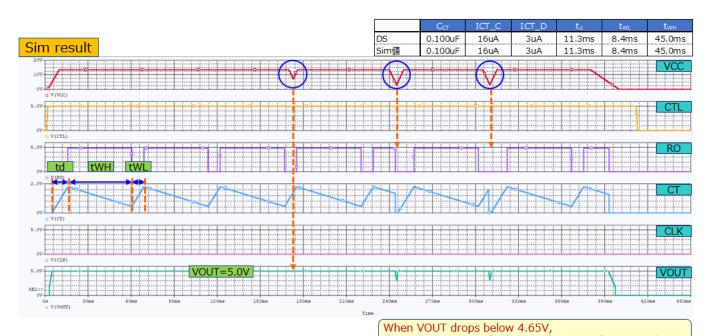
the reset operation discharges the CT and negates the RO
