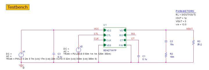
When output control voltage VCTL is ON ⇔ OFF (Input=13.5V Output=5.0V IOUT=1pA)
