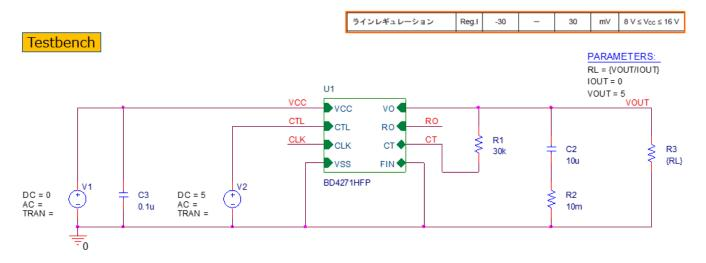
Line regulation (Input=8V~16V Output=5.0V IOUT=0A)
