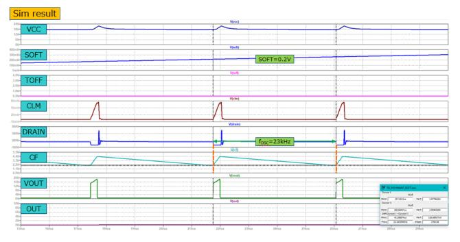
Oscillator operation at the SOFT(Input=138V Output=8.5V IOUT=1.0A)
