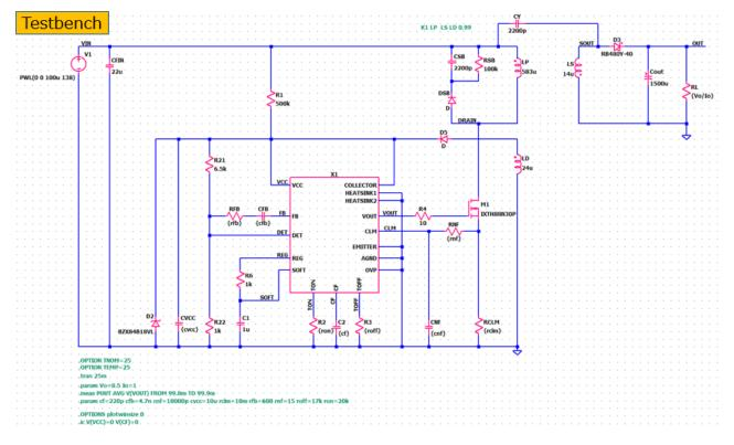
Oscillator operation at the SOFT(Input=138V Output=8.5V IOUT=1.0A)
