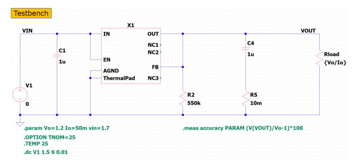
Line regulation (Input=1.5V~6V Output=1.2V IOUT=50mA)
