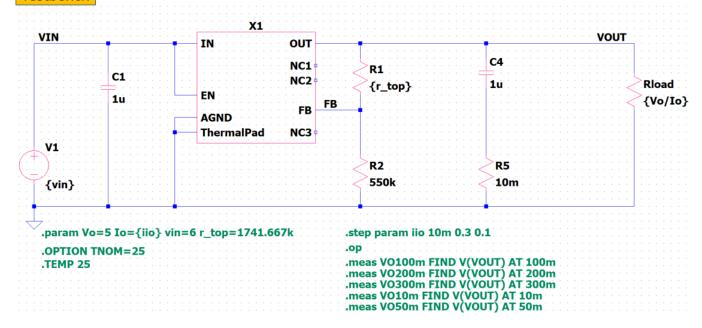
Load regulation (Input=6V Output=5.0V IOUT=10mA~0.3A)
