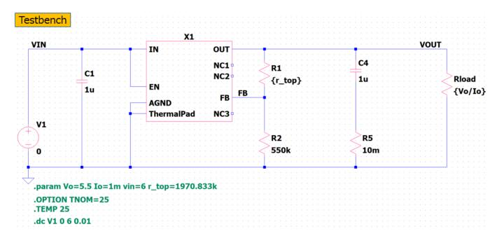
Output Voltage vs Input Voltage (Input=0V~6V Output=5.5V IOUT=1mA)
