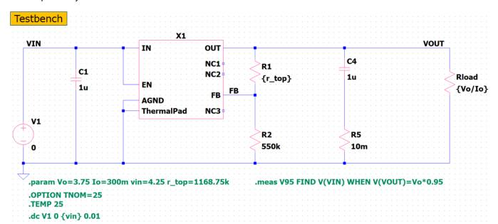
Low-Dropout Voltage (Input=0V~4.25V IOUT=0.3A)
