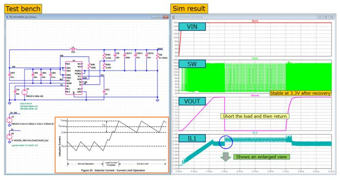
Valley Current Limit(Output=3.3V IOUT=2.5A) Simulation results are following.
