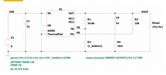
Line regulation (Input=0V~6V Output=3.3V IOUT=1mA)
