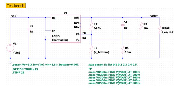
Load regulation (Input=3.8V Output=3.3V IOUT=0.1A~0.5A)
