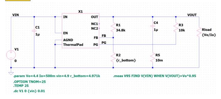
Low-Dropout Voltage (Input=0V~4.9V IOUT=0.5A)
