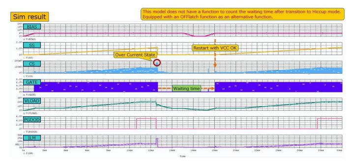
Overcurrent Protection(Input=12V Output=5.0V IOUT=2.1A⇒5.0A⇒2.1A)
