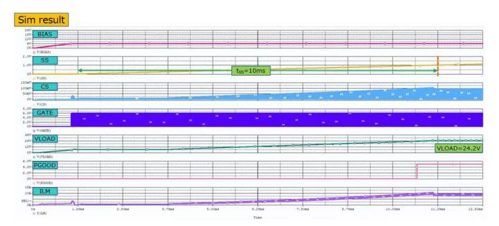
PWM Operation(Input=6V Output=24V IOUT=2A)
