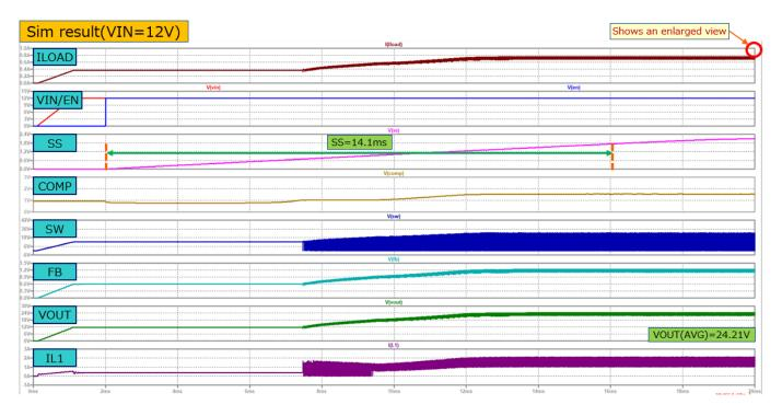
Boost Fixed frequency current mode PWM control(Input=12V Output=24V IOUT=0.75A f<sub>SW</sub>=603kHz) Simulation results are following.
