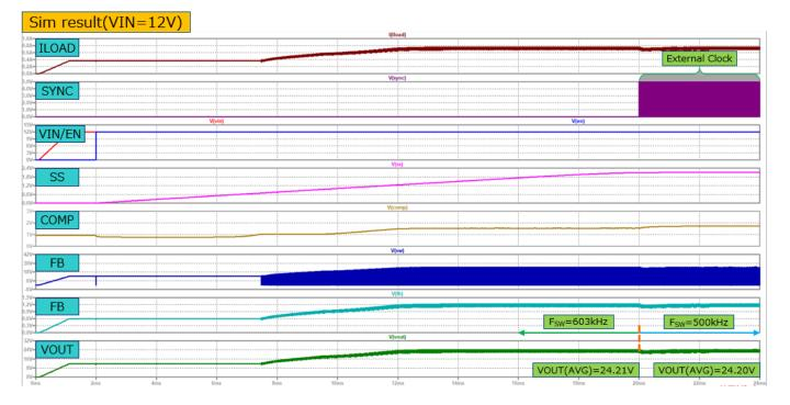
Boost Synchronization capability to external clock (  $f_{SW}{=}603kHz$  EX\_f\_{SW}{=}500kHz )
