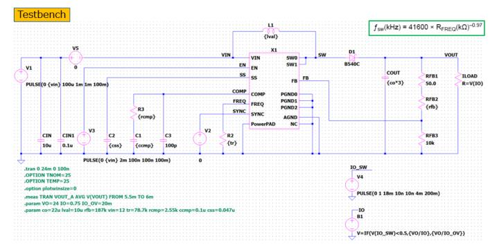
Boost Pulse skipping (Input=12V Output=24V IOUT=0.75A⇒0.02A⇒0.75A) f<sub>SW</sub>=603kHz
