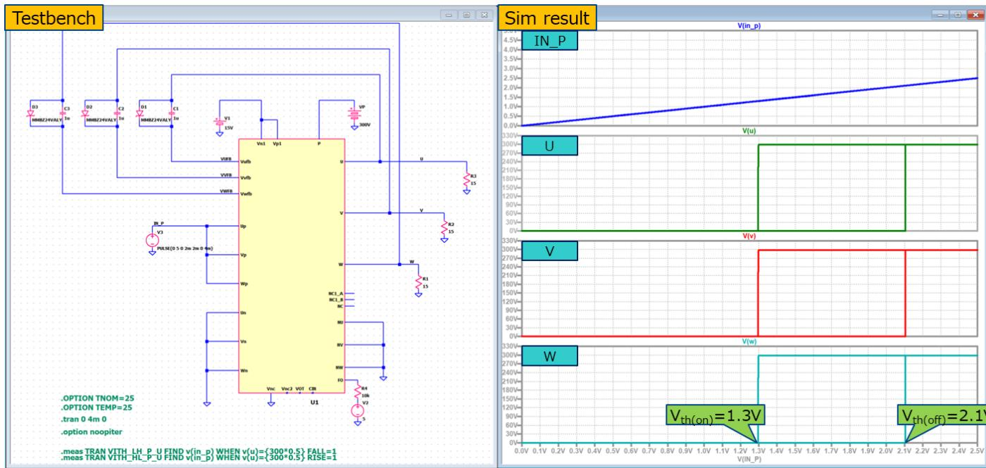
Input ON/OFF threshold voltage(N-side)
