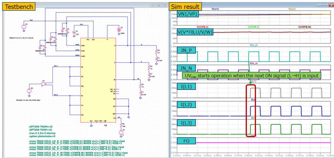
Undervoltage (UV) protection circuit (for P-side IGBT)
