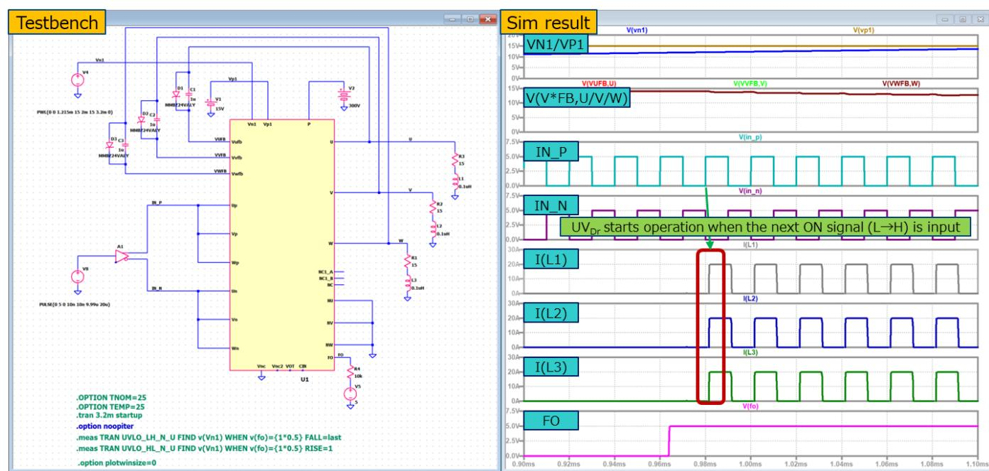
Undervoltage (UV) protection circuit (for N-side IGBT)
