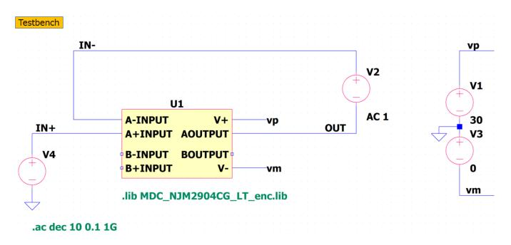
Open Loop Gain Simulation results are following. Explanatory notes — : simulated
