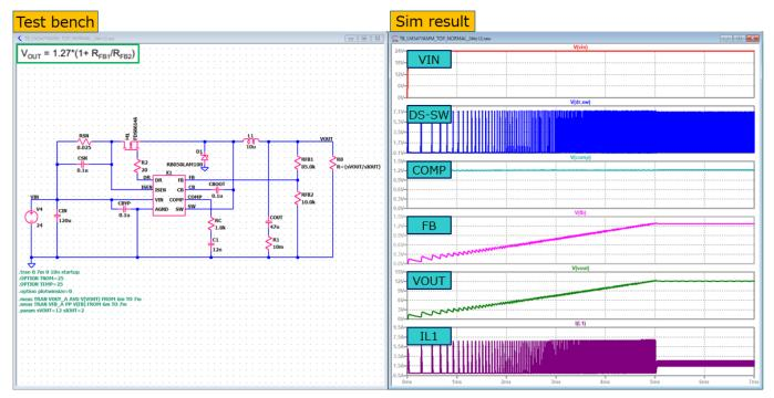
Current Mode Operation(Input=24V Output=12V IOUT=2A)
