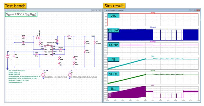
Over Voltage Protection(Input=12V Output=3.3V IOUT=3A⇒10mA⇒3A)
