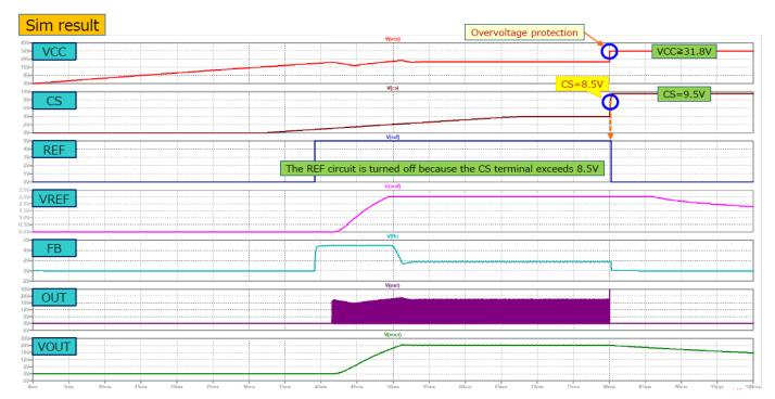
Overvoltage protection function detecting the Vcc voltage(Input=141V Output=24V IOUT=1.0A f<sub>SW</sub>=77kHz)
