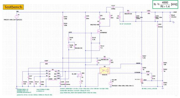
Output ON-OFF function by external signal (Input=141V Output=24V IOUT=1.0A f<sub>SW</sub>=77kHz)
