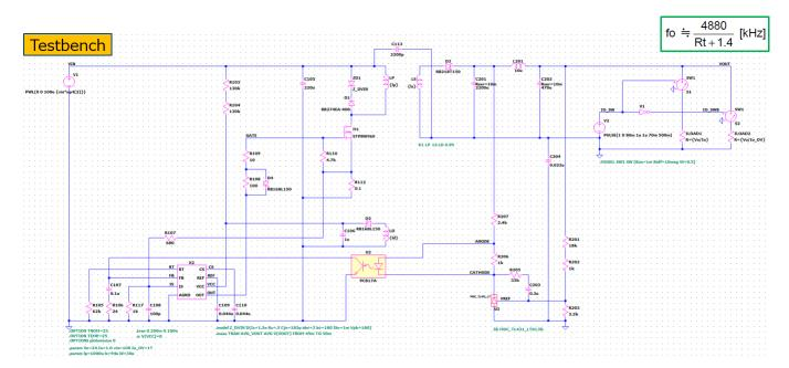
Overload protection function (Input=141V Output=24V IOUT=1.0A f<sub>SW</sub>=77kHz)
