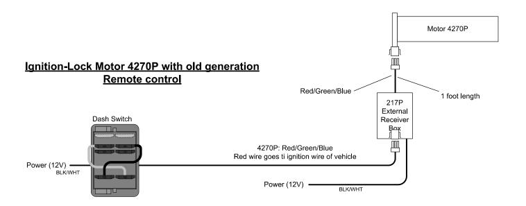
Note: This external Conversion Module 217P is only to be used with old generation AMS RF Remote Transmitters.
