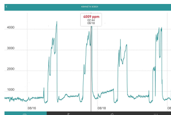
A readout from the device Jeremy Chrysler sent to school with his 13-year-old daughter. It reported CO2 levels above 4,000 p.p.m. when the school’s HVAC system was broken. via Jeremy Chrysler
