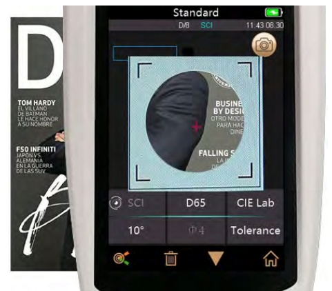
9. Camera framing and positioning can clearly observe the measured area
