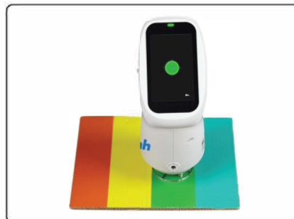
8. The camera can clearly observe the measured area
