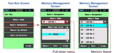
3. Align a memory in the selected memory name with the background blue position using the one-step icon or scroll bar.
