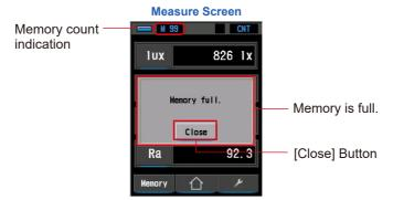
Return to the Measure Screen by touching the [Close] Button. To save the measurement value, delete the memory using [Memory Clear] and then try saving again. (▶ P66)
