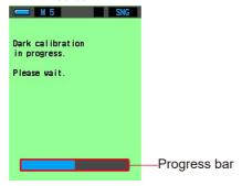
3. When dark calibration is finished, the Tool Box Screen is redisplayed.
