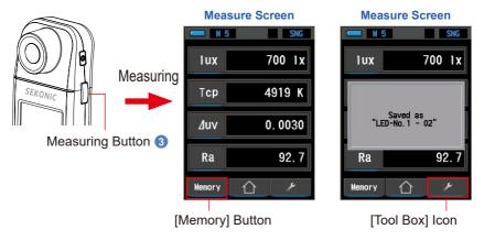
8. If you touch the [Save] Button on the Measure Screen, "Saved as" is displayed. The measurement values are saved and linked to the entered memory name.
