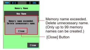
Touch the [Close] Button to return to the Memory Name Screen. To create a new memory name, delete unnecessary names from the Memory Management Screen and then try again. (→ P68)
