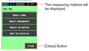
The setting is reflected on the status bar, and the measuring method is set.
