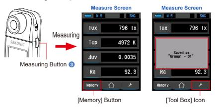
7. If you touch the [Save] Button on the Measure Screen, "Saved as" is displayed. The measurement values are saved and linked to the entered memory name.
