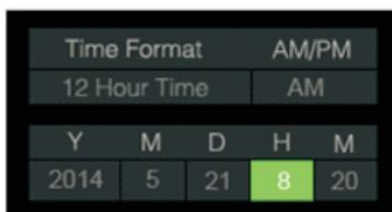
Unit can be set for the following: Time format (12 hours or 24 hours), AM/PM, date and time. Short press Up/Down key to change time settings, and short press ON/OFF/ENTER key to confirm, after confirming all settings, the unit returns to the main menu of settings screen.
