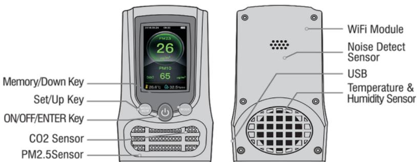
**Set/UpKey:** Long press to enter/exit the settings screen; Short press to switch measurement displaying on screen, or to scroll up in settings/memory screen.
