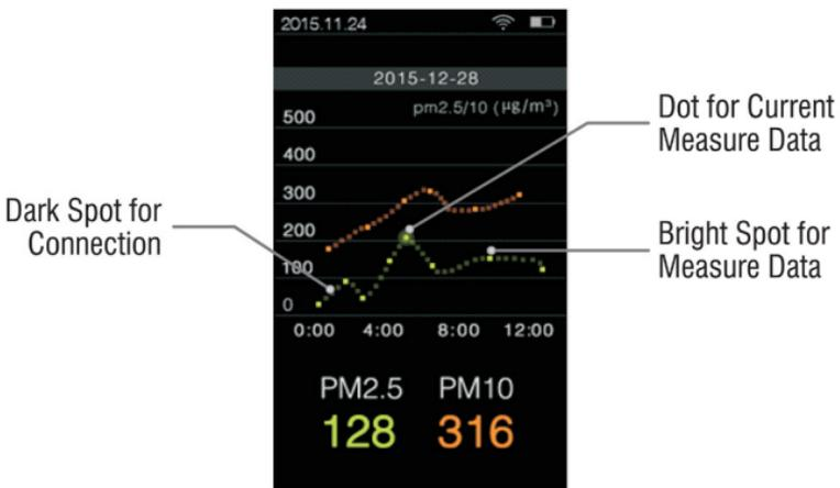
On measure screen, Long press MEM/DOWN key to enter/exit memory screen. Memory screen will dynamically display the latest curve of measurement data. To view the static measurement data, you can short press ON/OFF/ENTER key. On static memory screen, the device will display static curve of measurement data, and you can short press Up/Down key to view the detail of historical data one by one.
