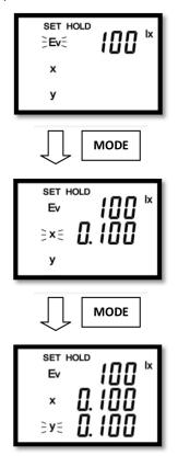
b. Using the measured values to set the reference values of ( $\triangle Ev$ ,  $\triangle u'$ ,  $\triangle v'$ ) mode.
