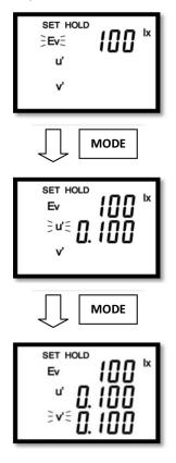
c. Using the measured values to set the reference values of ( ∠Ev, ∠CT, ∠u'v') mode.(522)
