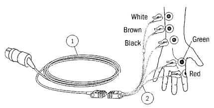
Figure 18-5. NMT setup with ElectroSensor
