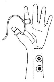
Figure 18-6. MechanoSensor attachment
