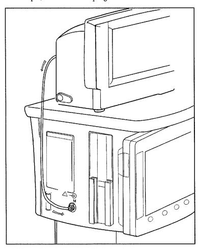
Figure 16-9 Connecting sample gas outlet directly to a anesthesia gas scavenging system
