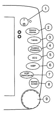
Figure 2-1. Cardiocap/5 keys and controls
