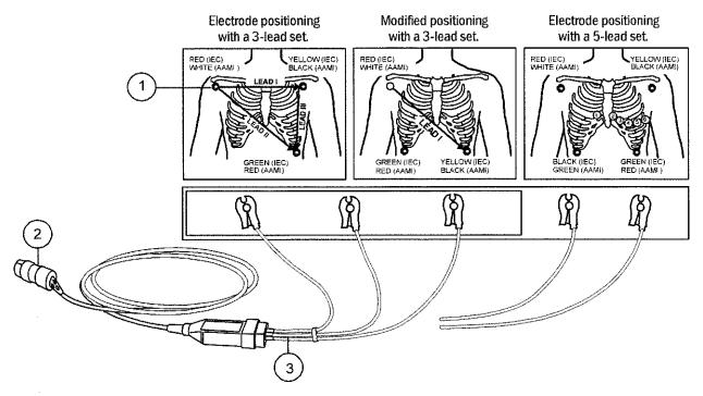
Figure 11-4. Impedance respiration setup
