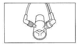
To prevent condensed water from entering the lines, position the gas sampling line and the spirometry tube connections so that they head upward from the patient.
