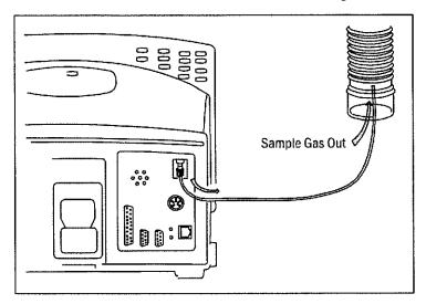
Figure 16-8. Scavenging through ventilator reservoir
