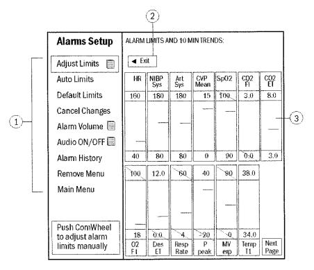
Figure 4-2. Alarms Setup menu and limits screen
