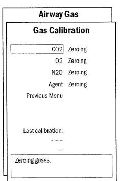
7. Wait until the "Zero ok" and then "Feed gas" messages appear on the screen after each gas.
