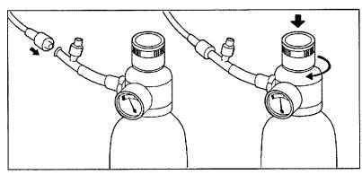
Figure 16-12. Connecting a sampling line to the gas valve and feeding gas
