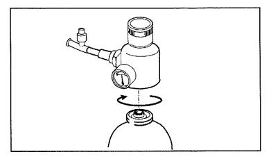
Figure 16-11. Attaching the regulator to the gas container
