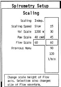
Figure 17-8. Vol Scale, Paw Scale, and Flow Scale options
