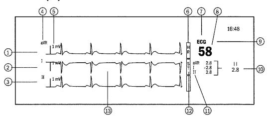
Figure 10-1. ECG and HR display
