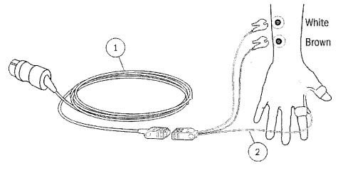
Figure 18-7. NMT setup with MechanoSensor
