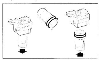
Figure 9-1. Emptying the water trap container
