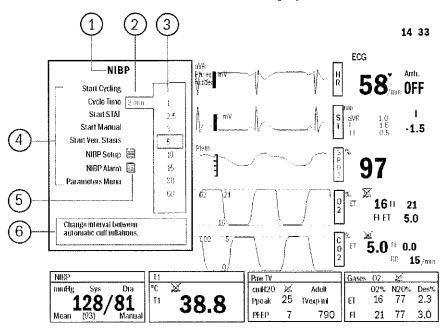
Figure 2-3. Parts of a menu
