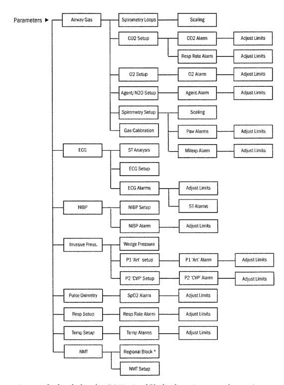
\* Menu is displayed when the NMT Regional Block Adapter is connected to monitor.
