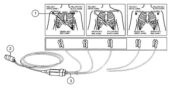
Figure 10-5. ECG setup
