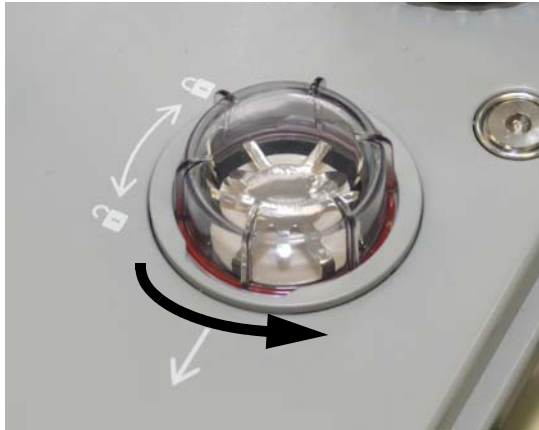
FIGURE 7-11 Valve Dome Removal
