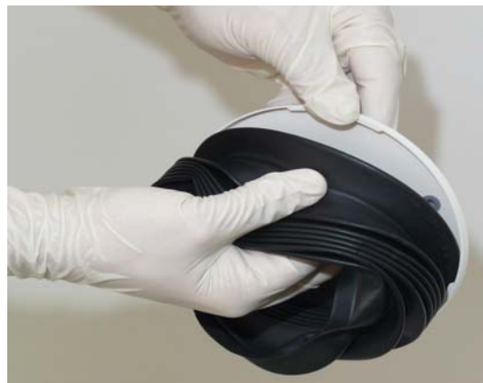
FIGURE 7-7 Detaching the Bellows Top Plate
