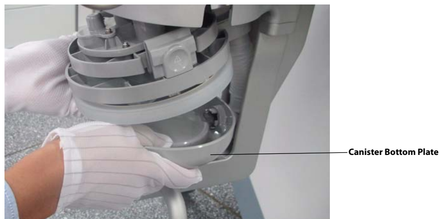
FIGURE 7-23 Remove Canister Bottom Plate
