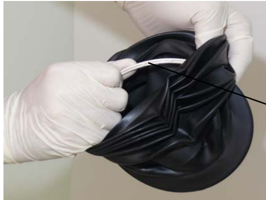
FIGURE 7-8 Removing the Bellows Adapter Ring
