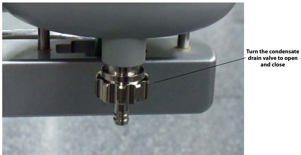
FIGURE 7-18 Condensate Drain Valve (Close Up View)
