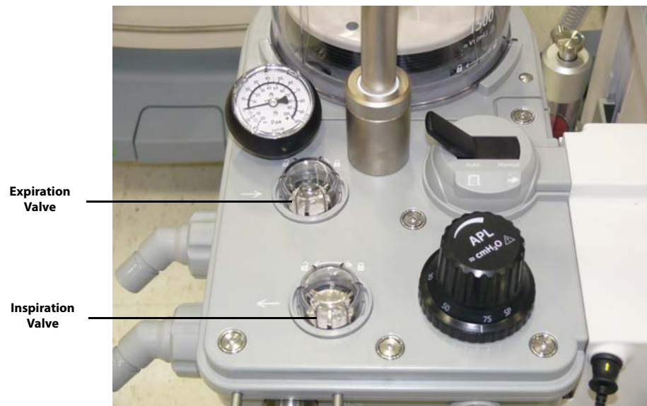
FIGURE 7-10 Location of Expiration and Inspiration Valves
