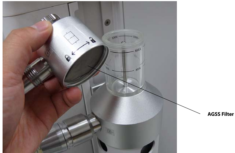
FIGURE 7-27 Removal of AGSS Top / AGSS Filter Inspection
