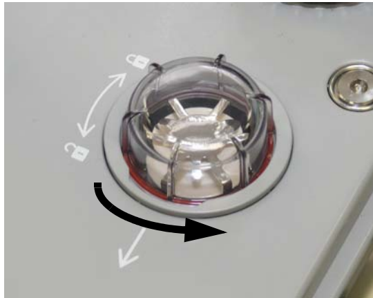
FIGURE 7-11 Valve Dome Removal
