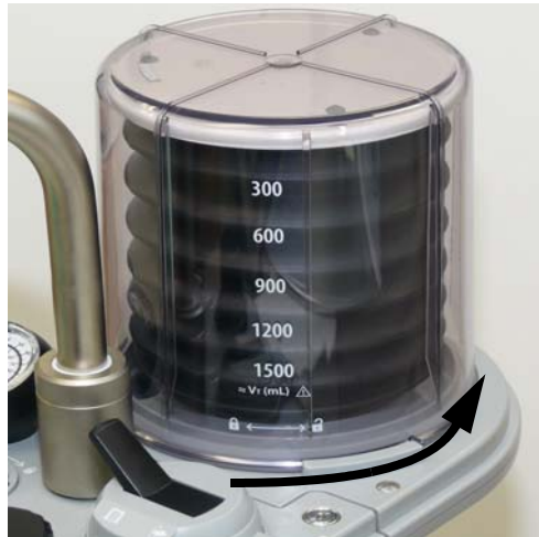
FIGURE 7-5 Removing the Bellows Dome
