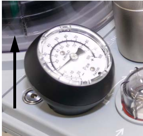
FIGURE 7-15 PAW Gauge Removal
