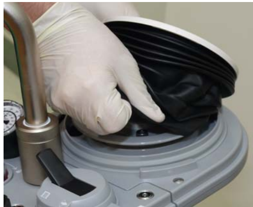
FIGURE 7-6 Detaching the Bellows
