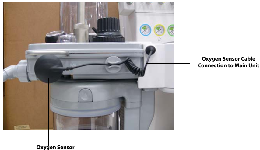
FIGURE 7-13 Oxygen Sensor and Cable
