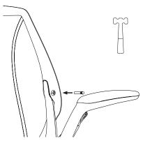
Install the back frame onto the seat frame using the 2 pins. Gently tap the pins using a mallet to securely seat the pins.
