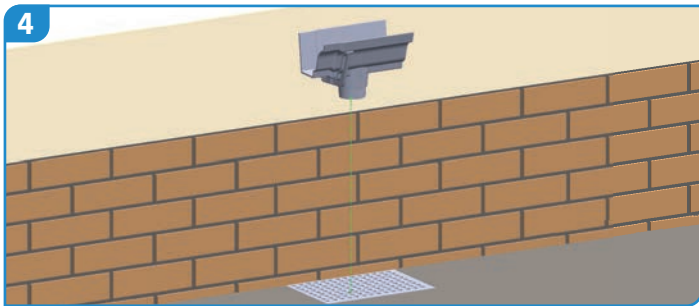
4 With the use of a plumb or laser line, position outlets over gullies and support with at least one bracket. Also include a bracket per angle (internal or external).
