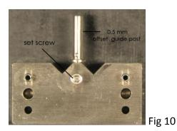
A *stylus* was placed over the upper portion of the guide post and the guide post was bent to the right to correct the first angle (Figure 8)).
