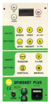
If at anytime the machine malfunctions, turn off the power switch to reset the machine's control logic. In most circumstances, the improper working of the machine is caused by low battery voltage. In this case, please recharge your battery to resume normal operation.
