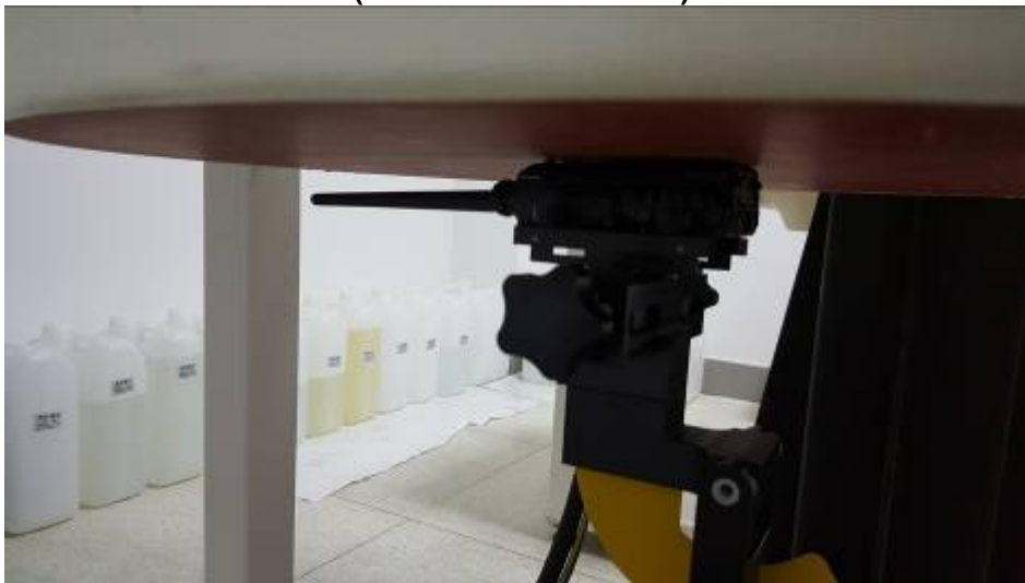
Body-worn, the front of the EUT towards phantom (The distance was 0mm)
