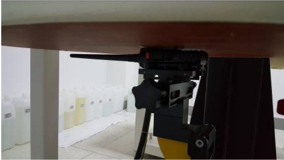
Body-worn, the front of the EUT towards ground (The distance was 0mm)
