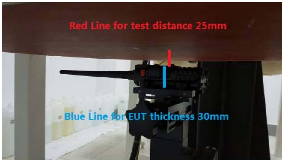
Face-held, the front of the EUT towards phantom (The distance was 25mm)
