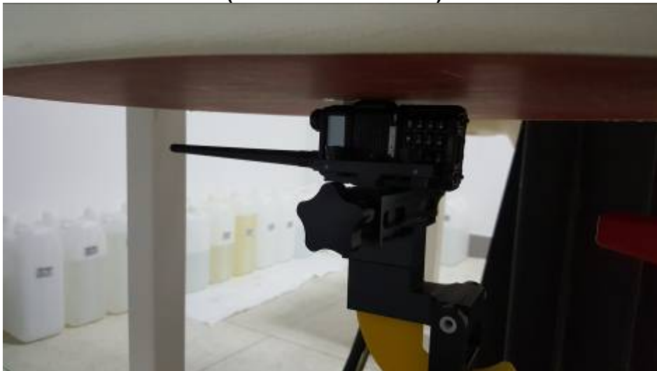
Body-worn, the right of the EUT towards phantom (The distance was 0mm)
