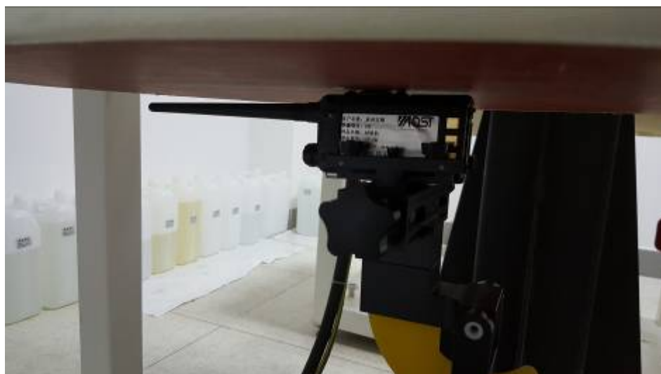
Body-worn, the left of the EUT towards phantom (The distance was 0mm)
